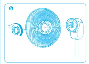
5.使用網鎖把後網鎖緊在電機外殼前面。 Fixing the rear guard onto the front of motor housing by the guard cap.
