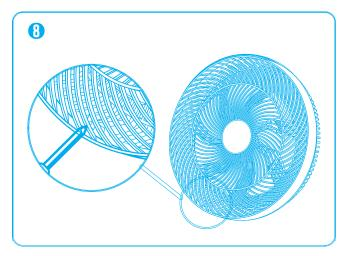
8.將後網下方螺絲鎖緊。 Fix the rear guard with the screw.
