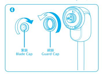
4.從電機軸取出葉鎖及網鎖。 Remove the blade cap and guard cap from the motor shaft.
