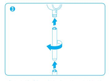
3.把主機體插入外柱中,並順時針旋轉 主機體將主機體鎖緊在外柱。 Insert the main body into the outer pole and rotate the main body clockwise to lock the main body to the outer pole.
