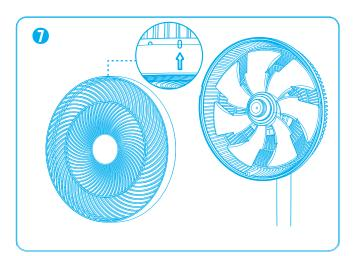
7. 把前網放在後網上,順時針旋轉前網。 Put the front guard onto the rear guard, turn the front guard clockwise.
