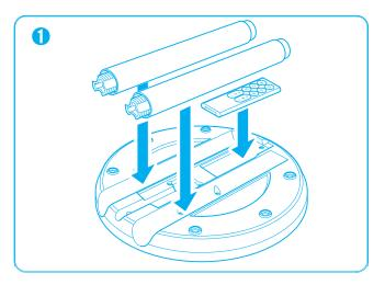
1.從底座底部取出兩條外柱及遙控。 Take out the two outer poles and remote control from the bottom of the base.
