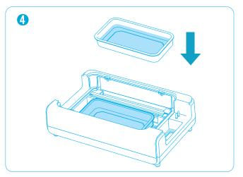
4. 然後將水盤放在底座底部。(注意: 注水時切勿將水滴到發熱線上。) Place the water tray in the bottom of the base. (Note: Please do not drip water onto the heating element.)
