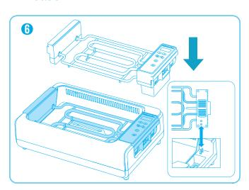
6. 將發熱線放在底座上,對準發熱線 上與底座上的安全切斷開關。 Place the heating element on the base, aligning the safety cut off switch on the base with the safety cut off switch on the base.
