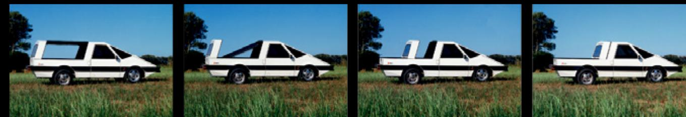
LOGICAR | DESIGN STUDY | 1982 | TOP: SCALE 1:1 MODEL | BELOW: FULL SIZE WORKING PROTOTYPE: CONVERSION FROM AN ESTATE CAR TO PICK-UP
